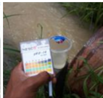
Kegiatan Penyiraman Jalan Tambang Measurement of water quality (pH) at SP outlet
